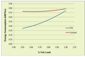
System differences in efficiency between a constant speed chiller compared with that of a VFD operated chiller
